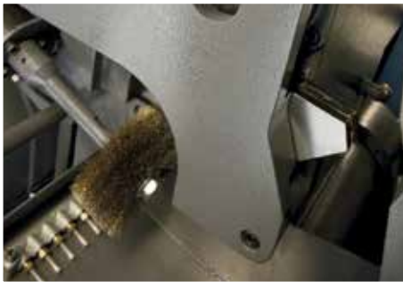
Power driven chip brush actively cleans chips from the saw blade. This extends blade life and maintains cutting efficiency.
