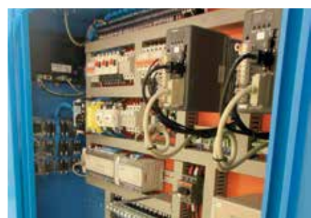
Split door of TC-155NC for easy access to different parts of the machine to improve maintenance control.
