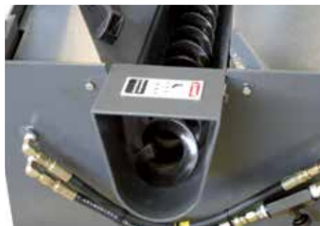
Automatic chip conveyor
