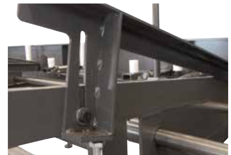
Automatic loading table efficiently moves round material only from the loading area to the infeed area.
