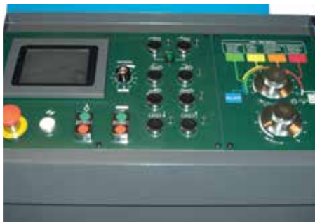
Color touch screen control panel and manual buttons NC-models
