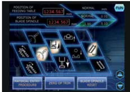
Touch screen and control panel allow easy operation. The information for problem solving & trouble shooting is shown on the screen and historical data is recorded for reference.
