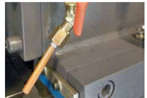
Cleaning nozzle to extend blade life.
