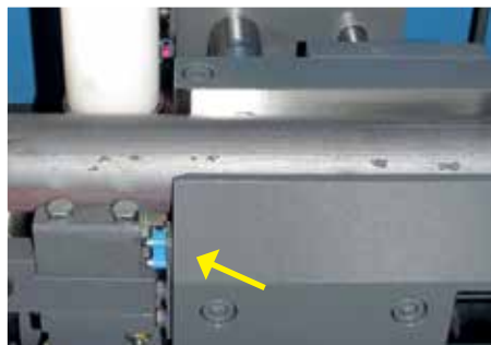
Optical sensor for increased reliability.
